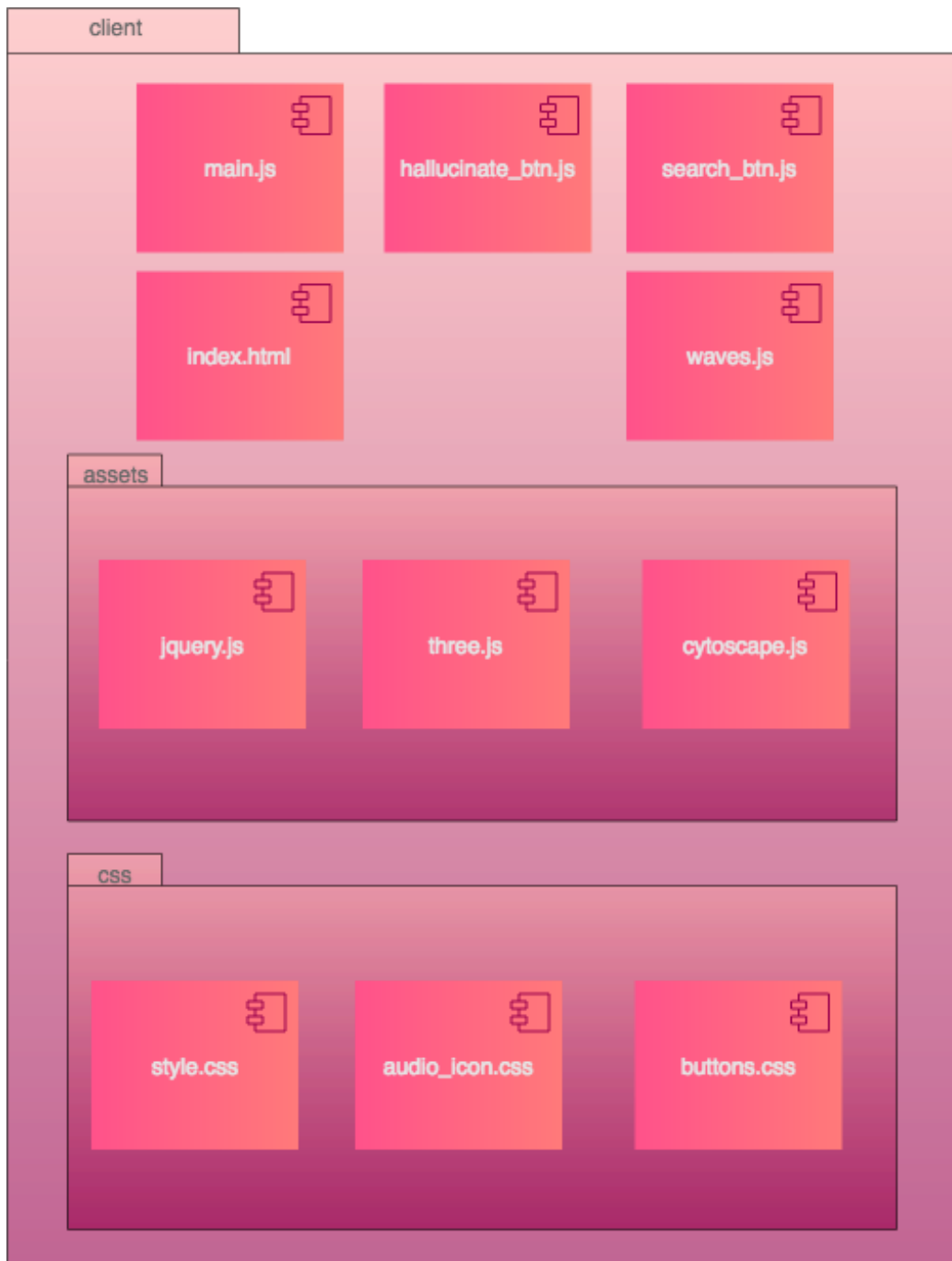
Figure 2 This is the UML diagram for the components and packages of the client side of Etymøn.
